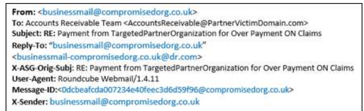
Figure 2: Email header showing attacker ability to receive all replied emails sent to unsuspecting senders.
